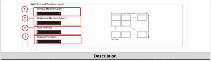
Provide the settings regarding the amount of displays in the video wall, and the position of displays. Typical video
