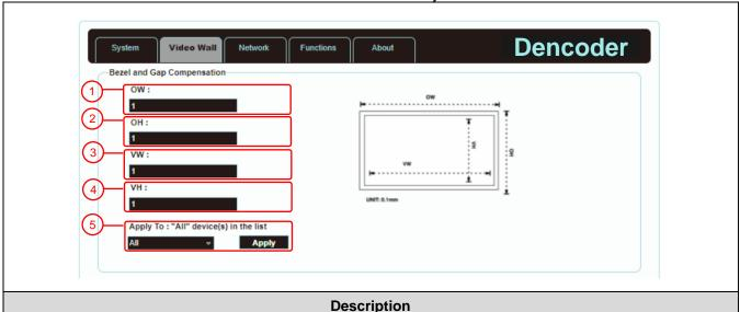
It provides the actual size setting of the display of the video wall. Various measurement units (inches, millimeters, centimeters) will do, as long as all measurements are in the same unit and the numbers are integers.
